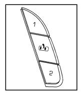
The controls for this feature are located on the driver door, and are used to program and recall memory settings for the driver seat, outside mirrors, and the adjustable throttle and brake pedal feature.
